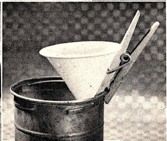
**FUNNEL CLIPS TO DEVELOPING TANK.** When a funnel is used for filtering developer, it can be attached to a spring clothespin which in turn can be clipped to edge of developing tank. The solution then will filter directly into container in which it will be used. Cellulose cement should be used to hold the funnel to the clothespin.
