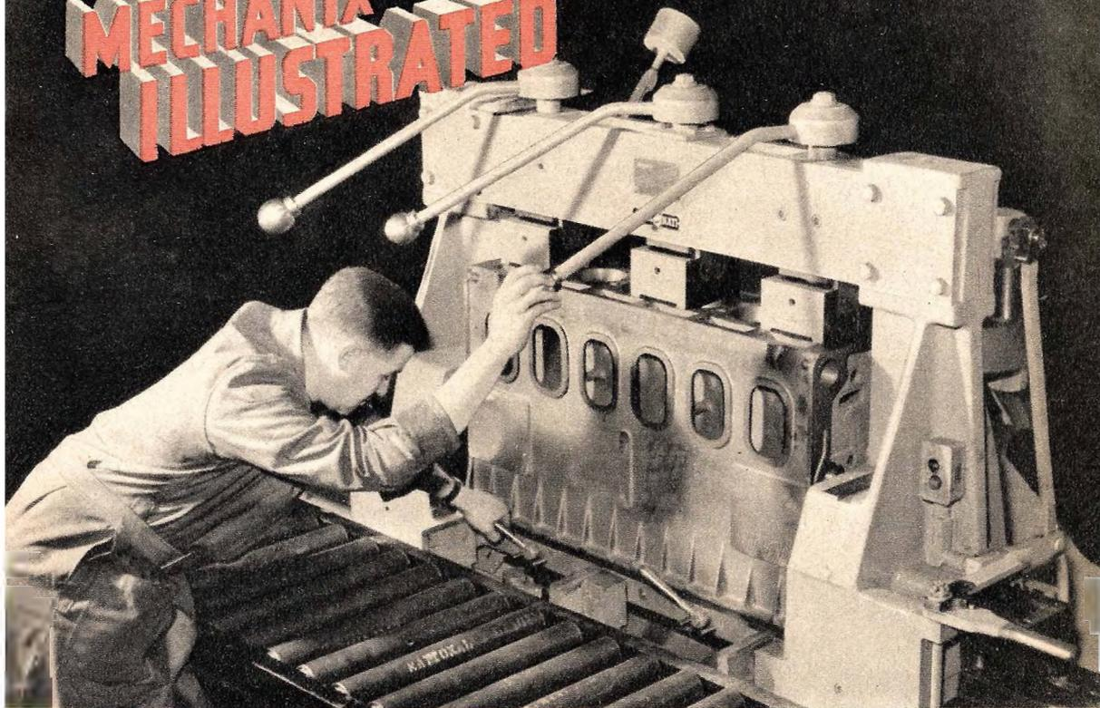
This machine cuts grooves in the diesel cylinder block.
