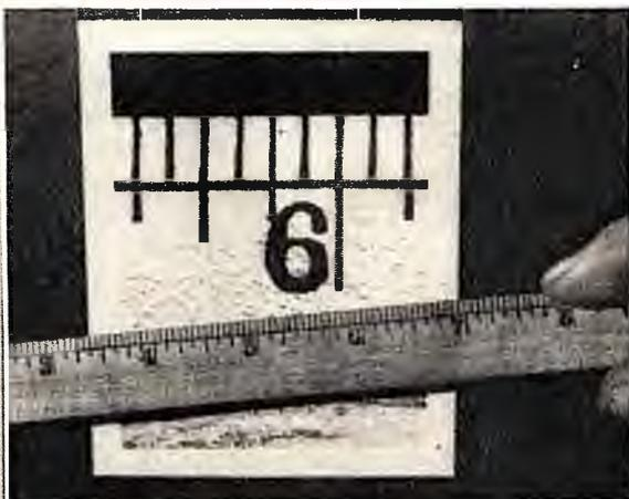
The marked degree of direct enlargement possible with the "close-up" camera is well illustrated in this picture. A 9 x 12 cm. contact print, made with the attachment, is compared with the actual size of the object, in this case a common ruler. Intimate close-ups of pins heads, nails, pebbles, grains of salt, etc., will suggest themselves to the ingenious photographer.
