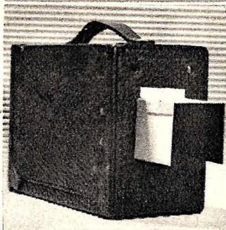
**SUN SHADE FOR BOX CAMERA.** A simple and inexpensive sun shade for a box camera can be made by cutting three 2-inch squares of cardboard and fitting it over the lens as shown in the photograph. The cardboard should be fastened together by narrow strips of adhesive tape.
