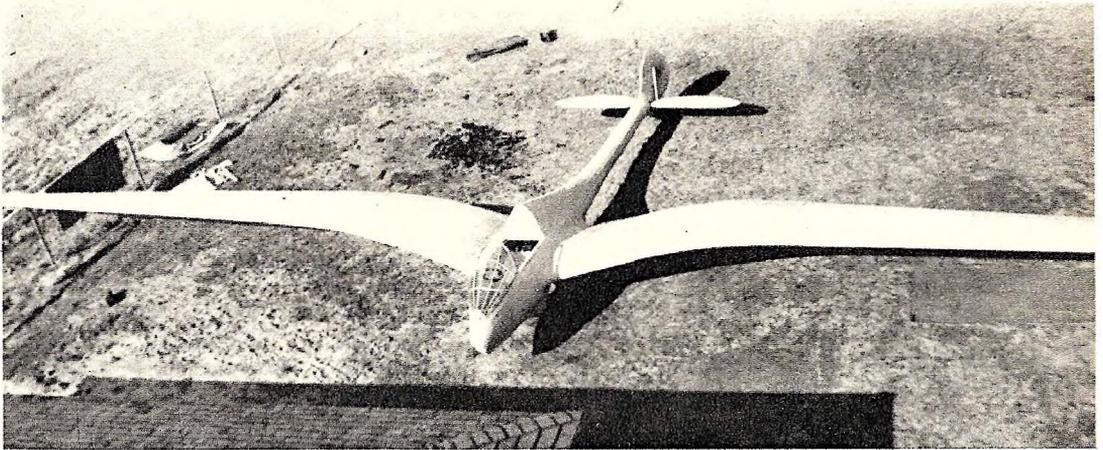
Featuring a full cantilever gull-type wing that gives it a truly bird-like appearance, a soaring glider constructed by Frank Merritt, of Glendale, Calif., has a wingspan of 72 feet and is believed to be the largest sailplane ever constructed in the
