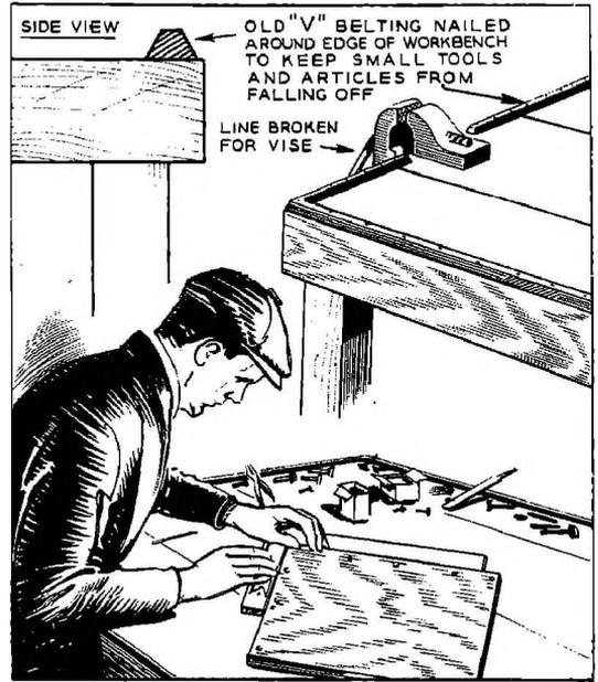
Ball bearings, small bolts and nuts, and other small articles have a tendency to roll off the workbench, falling to the floor to be stepped on, or lost. An old "V" fan belt tacked to the edge of the bench will prevent this from happening, and at the same time will not interfere with work. The narrow edge of the belt should face inside.—W. C. Wilhite.
